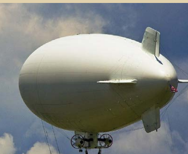
An optical fiber tether carries an analog ground radio signal to its corresponding antenna aboard the aerostat, providing greatly increased transmission range.
